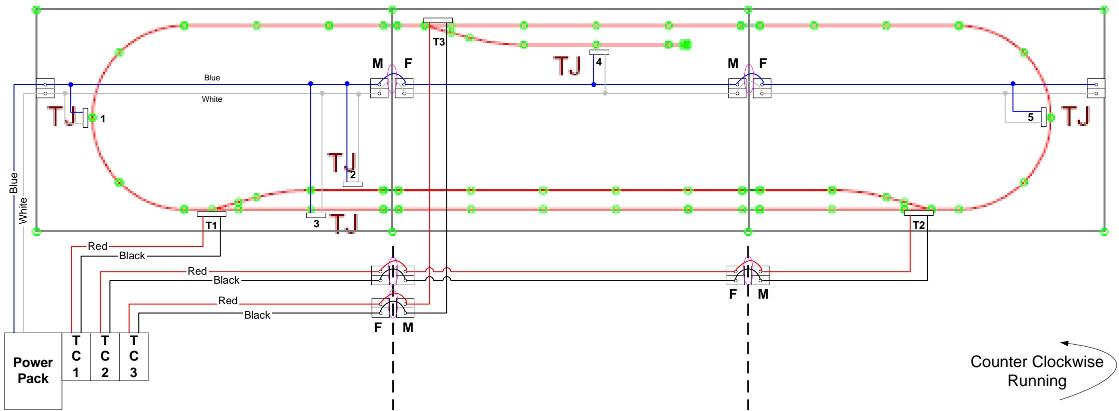
Track Power feeders are Blue & White (shown as Blue & Gray on diagram). There are five feeders numbered TJ1 through TJ5. Blue (-) is connected to the Inside Rail; White (+) to the Outside Rail. Turnout Power feeders are Red & Black. There are three turnouts numbered T1 through T3 that are controlled by turnout controllers TC1 through TC3.
